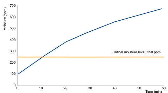
Figure 1: Moisture take-up curve semi-crystalline PLA
