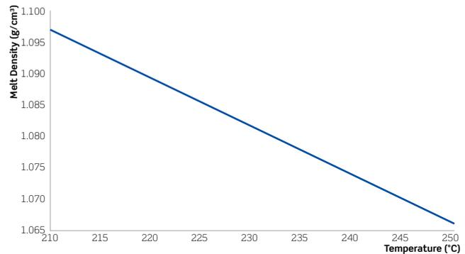
Figure 2: Melt Density as a function of temperature
